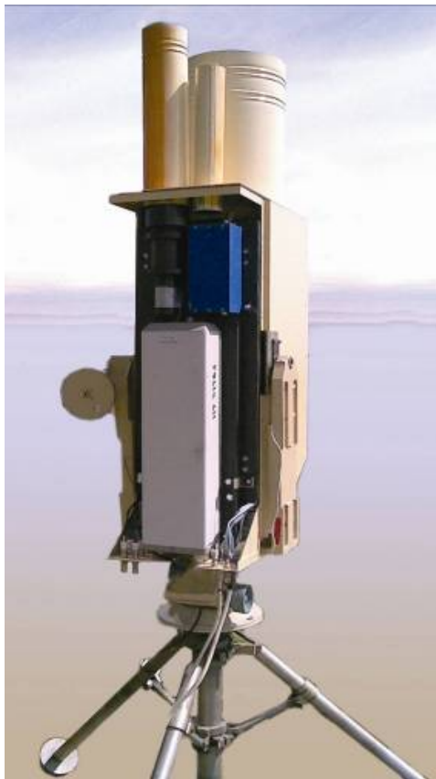
Aerosol lidar (IAO SB RAS) Monitoring of altitude profile of troposphere aerosol
