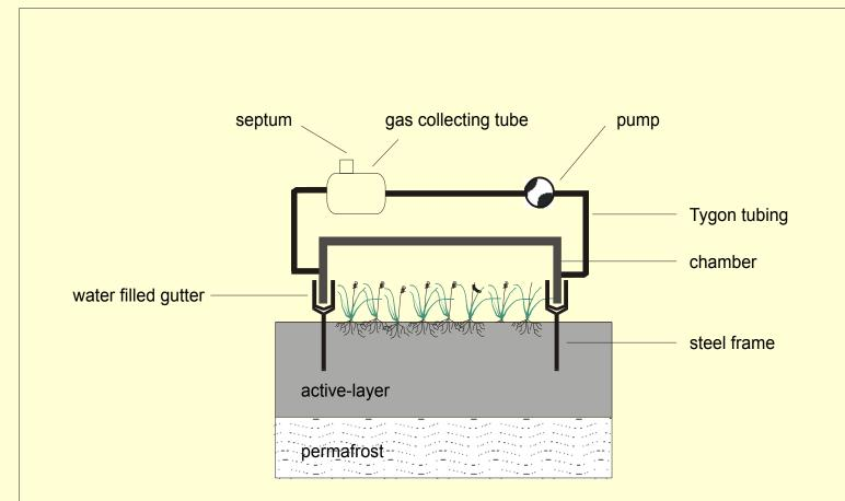
We used the method of closed chambers (Wagner et al., 2003) for fixing the methane released from the soil surface
