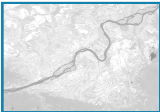
TIRS (Thermal Infrared Sensor ) 10, 11 bands Landsat 8 100 m
